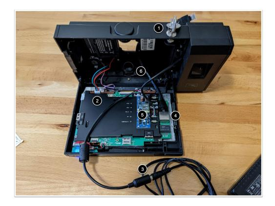
Inside your Time Machine there are multiple connections you'll want to ensure are connected properly:
